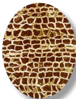
Radial section of cork cells. Naturally airtight and watertight.
